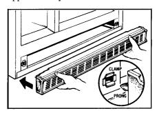
To replace base grille, align prongs on back of grille with clamps in cabinet and-push forward until the grille snaps into place.
